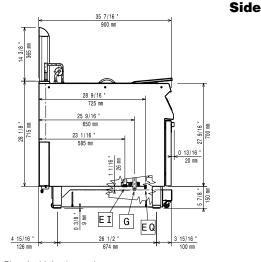
EI = Electrical inlet (power) Equipotential screw Gas connection
